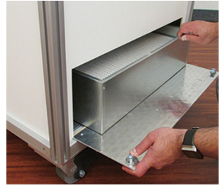
HEPA replacement via exterior door. Interlock on HEPA door to stop blower motor and turn off UVC/UVGI lights when opened.
