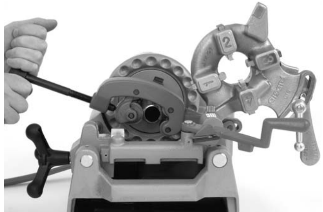
Figure 11 – Cutting Pipe with No. 354 Cutter
