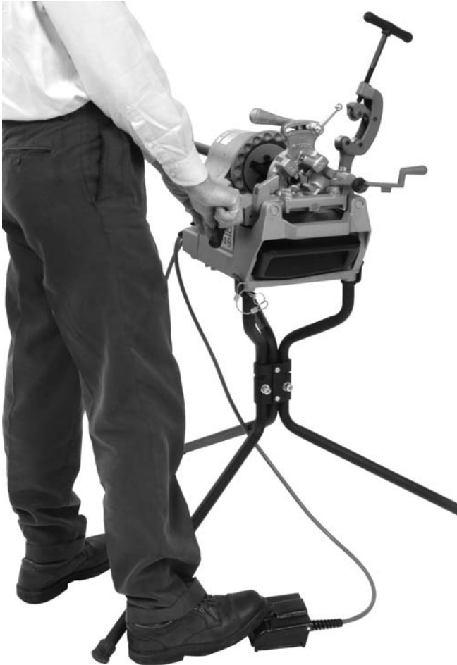
Figure 10 – Operator in a proper operating position
