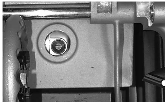
Figure 19 – Brush Cap Plug Removed, Brush Holder Exposed
