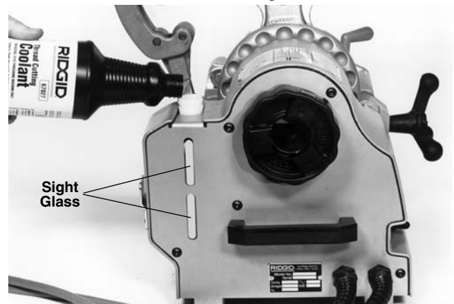
Figure 5 – Filling Coolant Reservoir
